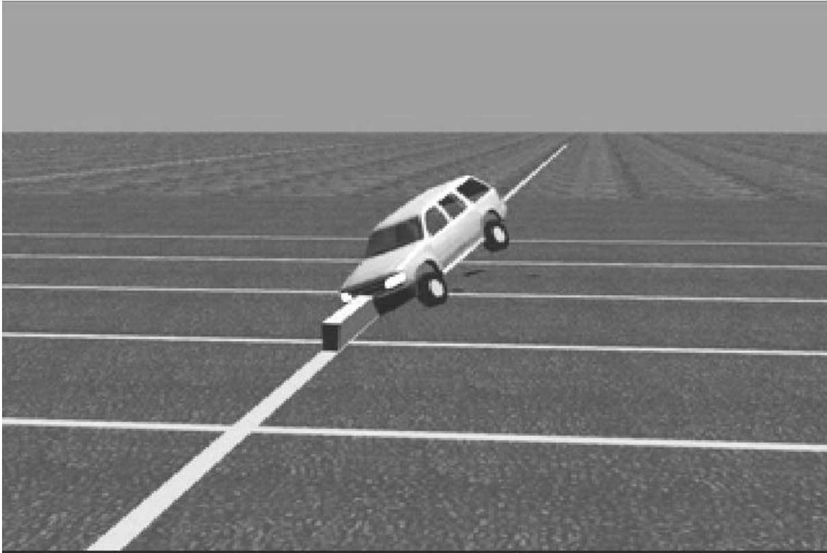
Figure 8 Clip from RTB barrier simulation for a 4WD at 80 km/h and 30 degree approach angle
