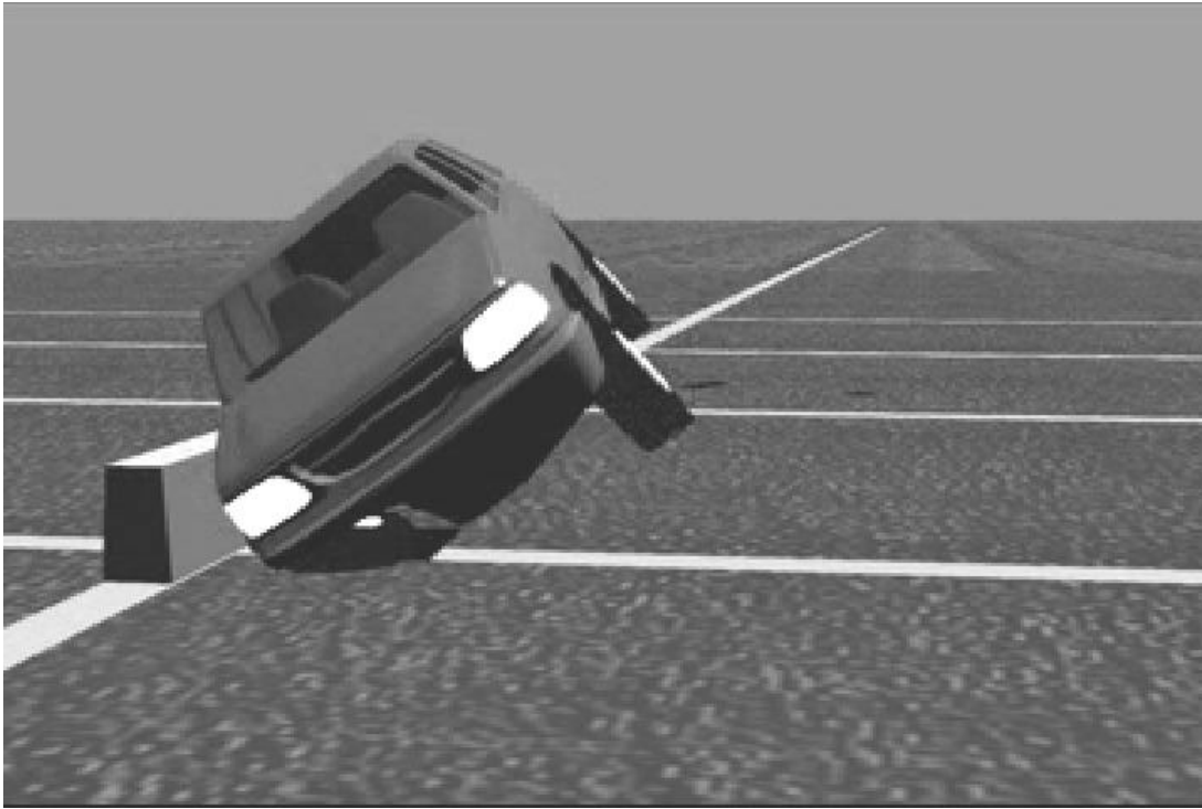
Figure 6 Clip from RTA barrier simulation for a 4WD at 80 km/h and 30 degree approach angle
