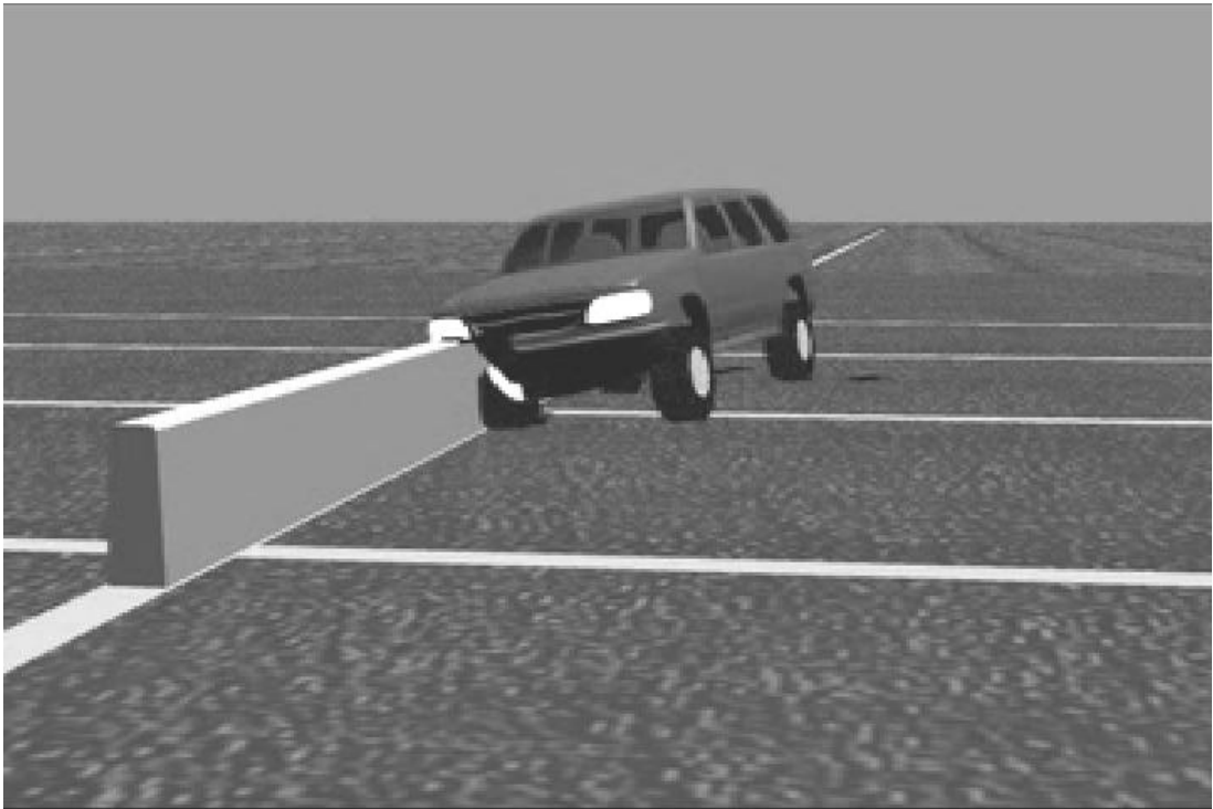
Figure 9 Clip from VCB barrier simulation for a 4WD at 80 km/h and 30 degree approach angle
