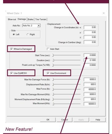
Start Time (sec) controls when the DyMESH wheel impact model is turned on. Auto Start will turn the DyMESH wheel impact model on when SIMON detects any impact with the vehicle.
