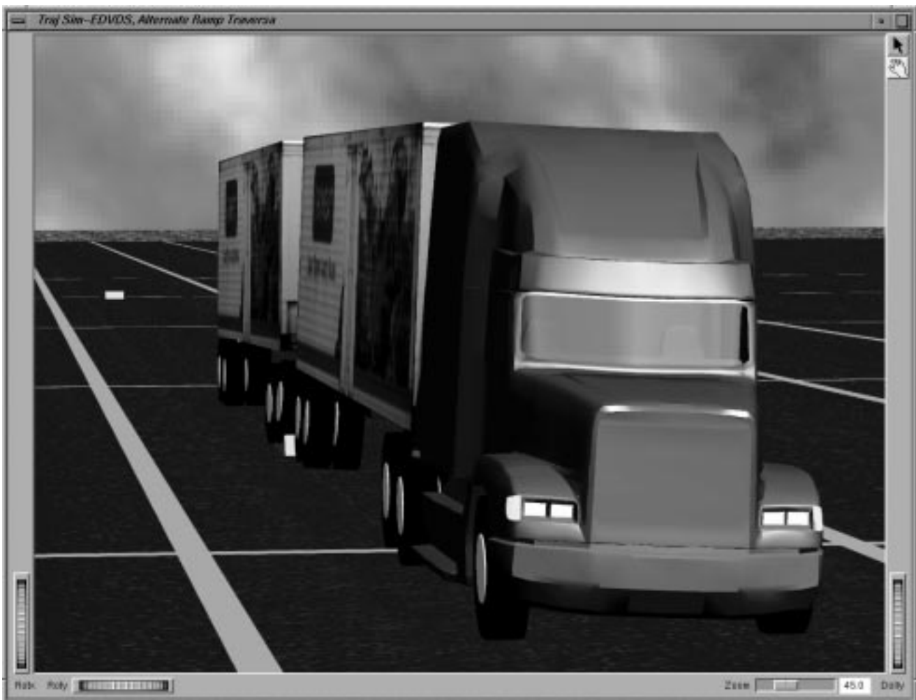
Figure 2 - HVE simulation environment with an EDVDS simulation of an alternate ramp traversal, used for studying the effect of torsional frame compliance on the handling and control of a set of highway doubles.
