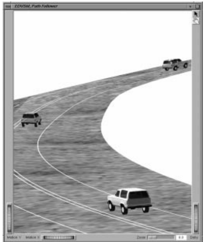
Figure 4 - Spline path definition for up to eight user-defined vehicle positions and orientations.
