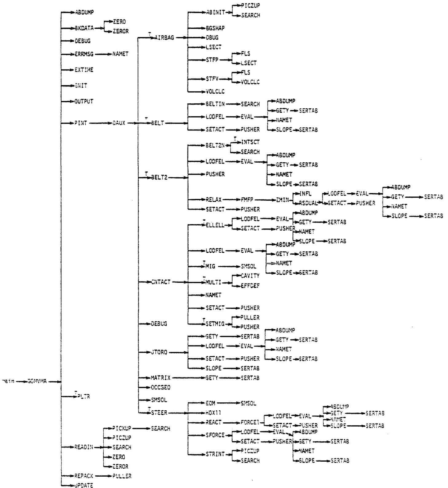
Figure 136. Calling Structure for the Dynamic Solution Processor (GO).
