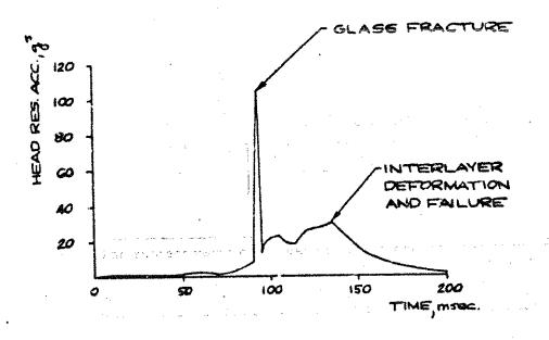
Figure 3.1.3 TYPICAL PREDICTED HEAD ACCELERATION RESPONSE
