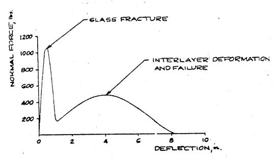
Figure 3.1.2 WINDCHIELD FAILURE CHARACTERISTIC
