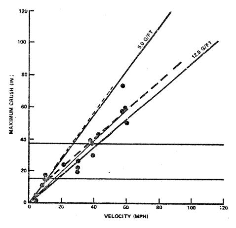
Figure C-1 FRONT IMPACTS WITH RIGID POLES (DATA POINTS FROM REF. 20)
