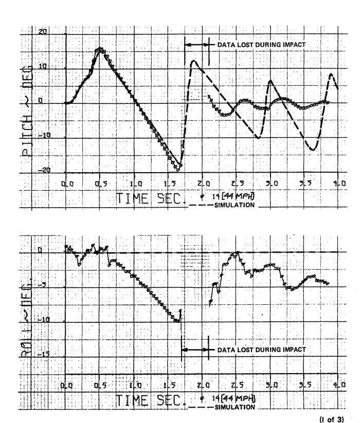
Figure 2.2-13 MEASURED AND PREDICTED RESPONSES OF VEHICLE JUMP FROM TAKE - OFF RAMP
