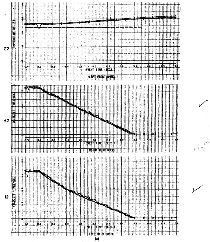
igure 2.6-4 (Cont.) COMPARISON OF MEASURED AND COMPUTED VEHICLE RESPONSES — CORNERING AND BRAKING MANEUVER
