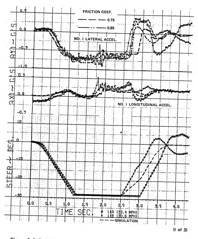
Figure 2.3-7 MEASURED AND PREDICTED RESPONSES OF VEHICLE IN REVERSE SKID ON DRY PAVEMENT
