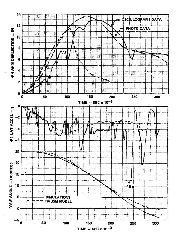
Figure 2.4-4 VEHICLE AND BRIDGE RAILING RESPONSES - TEST NO. 1
