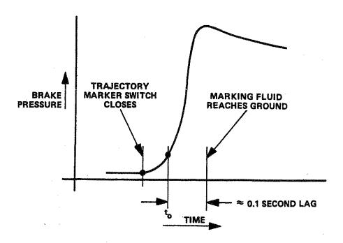
Figure 2.5-13 SEQUENCE OF EVENT RELATIVE TO TRAJECTORY MARKING
