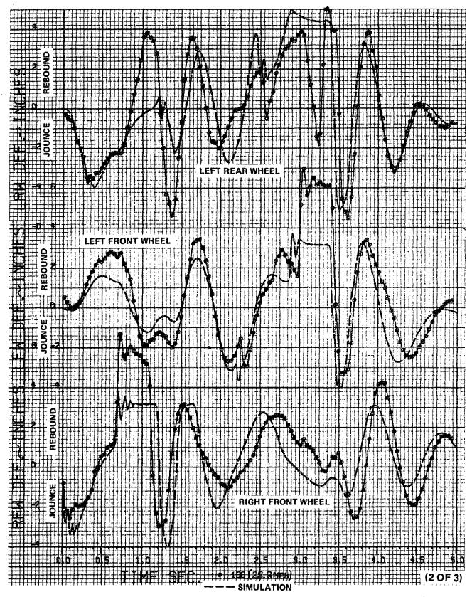
igure 2.2-11 MEASURED AND PREDICTED RESPONSES OF VEHICLE TRAVERSING 3.6° - 21.5" HIGH RAMPS ALTERNATELY WITH RIGHT AND LEFT WHEELS (TEST 13b) (continued)
