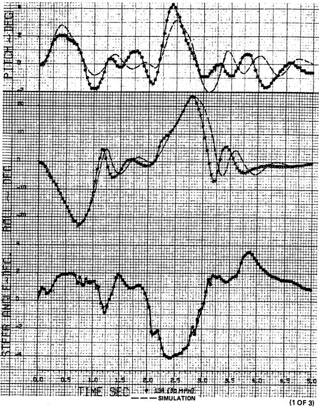
gure 2.2-10 MEASURED AND PREDICTED RESPONSES OF VEHICLE TRAVERSING 3.6° - 21.5" HIGH RAMPS ALTERNATELY WITH RIGHT AND LEFT WHEELS (TEST 13a)
