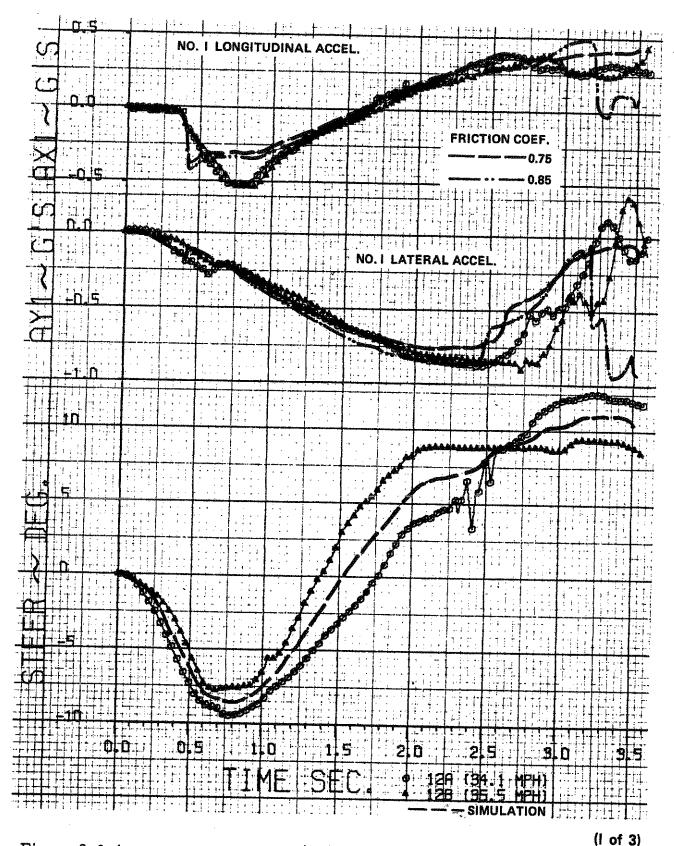
Figure 2.3-6 MEASURED AND PREDICTED RESPONSES OF VEHICLE IN FORWARD SKID ON DRY PAVEMENT
