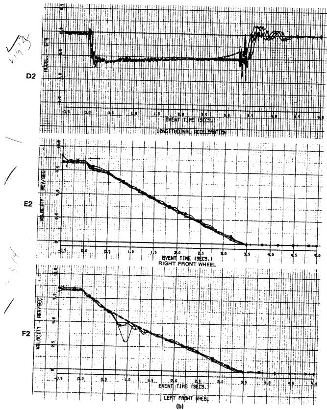
Figure 2.6-4 (Cont.) COMPARISON OF MEASURED AND COMPUTED VEHICLE RESPONSES — CORNERING AND BRAKING MANEUVER
