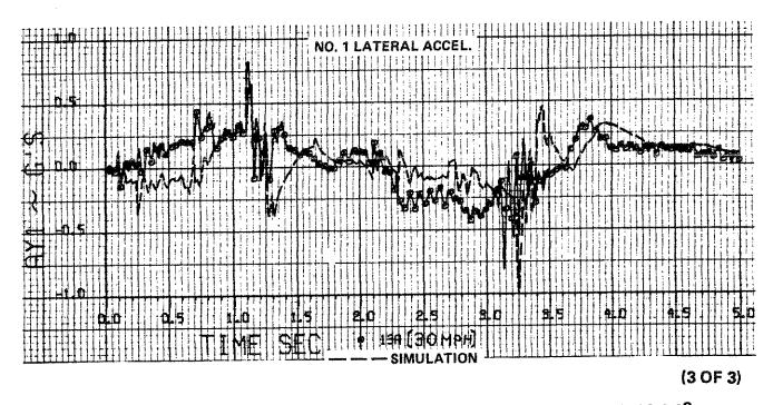
1Te 2.2-10 MEASURED AND PREDICTED RESPONSES OF VEHICLE TRAVERSING 3.6° - 21.5" HIGH RAMPS ALTERNATELY WITH RIGHT AND LEFT WHEELS (TEST 13a) (continued)
