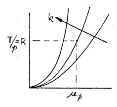
Thus, for the measured value of the torque coefficient,  $R = T/\rho$ , the required value of  $\mu_{\rho}$  is read off the curve for an assumed ratio  $k = \mu_{s}/\mu_{\rho}$ . Typically, the linings for Duo-Servo brakes are high coefficient on the primary shoe and low coefficient for the secondary shoe (Reference 3).
