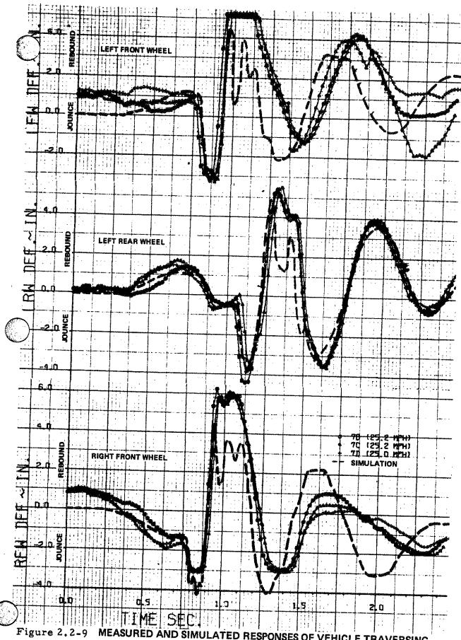
rigure 2.2-9 MEASURED AND SIMULATED RESPONSES OF VEHICLE TRAVERSING 7.10 — 6.75" HIGH RAMP WHILE CORNERING AT 0.4G (Continued)
