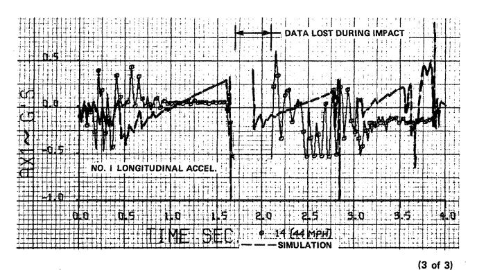
Figure 2.2-13 MEASURED AND PREDICTED RESPONSES OF VEHICLE JUMP FROM TAKE - OFF RAMP (continued)
