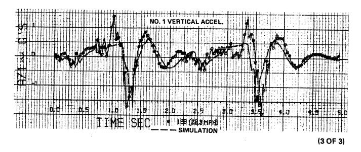
Figure 2.2-11 MEASURED AND PREDICTED RESPONSES OF VEHICLE TRAVERSING 3.6° - 21.5" HIGH RAMPS ALTERNATELY WITH RIGHT AND LEFT WHEELS (TEST 13b) (continued)
