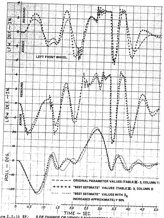
THE 2.2-15 EFF S OF CHANGE OF VEHICLE PARAMETERS ON PREDICTED RESPONSES FOR TERNATE RAMP TRAVERSAL SIMULATION
