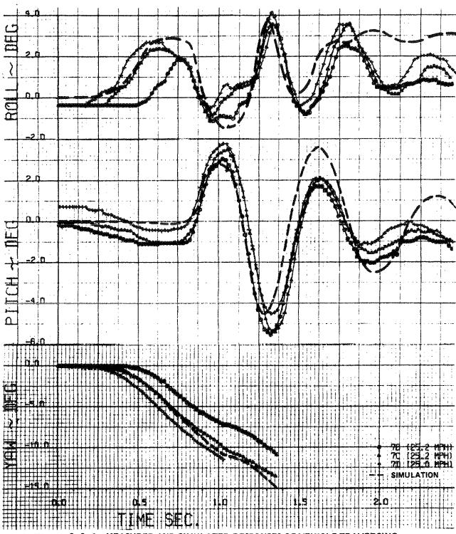
Figure 2.2-9 MEASURED AND SIMULATED RESPONSES OF VEHICLE TRAVERSING 7.1º — 6.75" HIGH RAMP WHILE CORNERING AT 0.4G (Continued)
