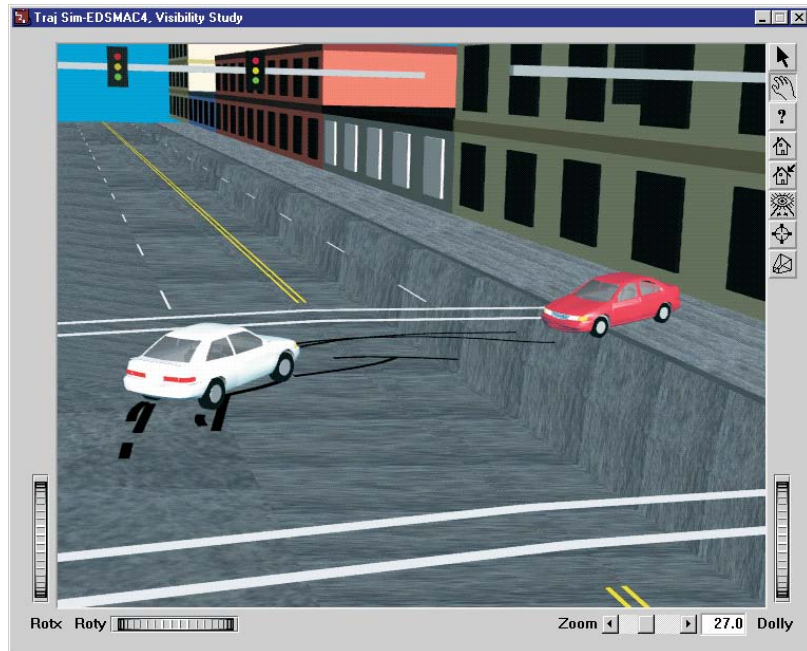
Figure 5-22 Trajectory Simulation for EDSMAC4, Visibility Study, displaying the crash sequence at the end of the event (HVE-2D, above, and HVE, below). Note, in the lower figure, the Nissan has come to rest on the sidewalk after mounting the curb.
