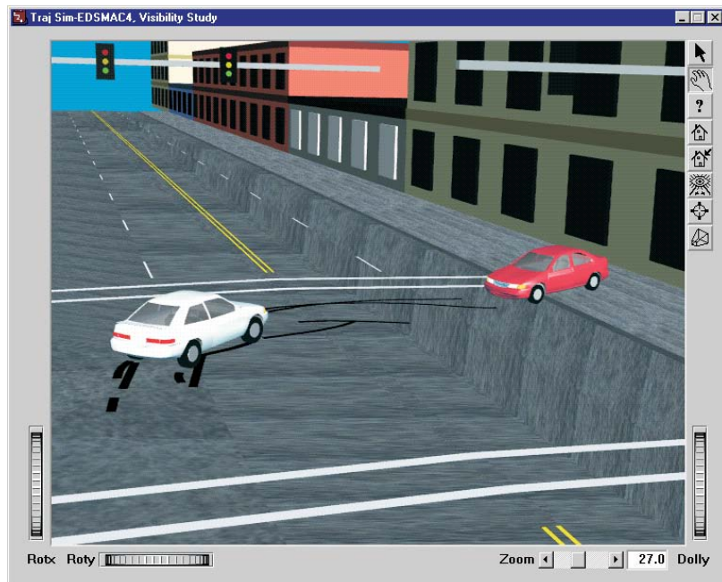
Figure 5-22 Trajectory Simulation for EDSMAC4, Visibility Study, displaying the crash sequence at the end of the event (HVE-2D, above, and HVE, below). Note, in the lower figure, the Nissan has come to rest on the sidewalk after mounting the curb.
