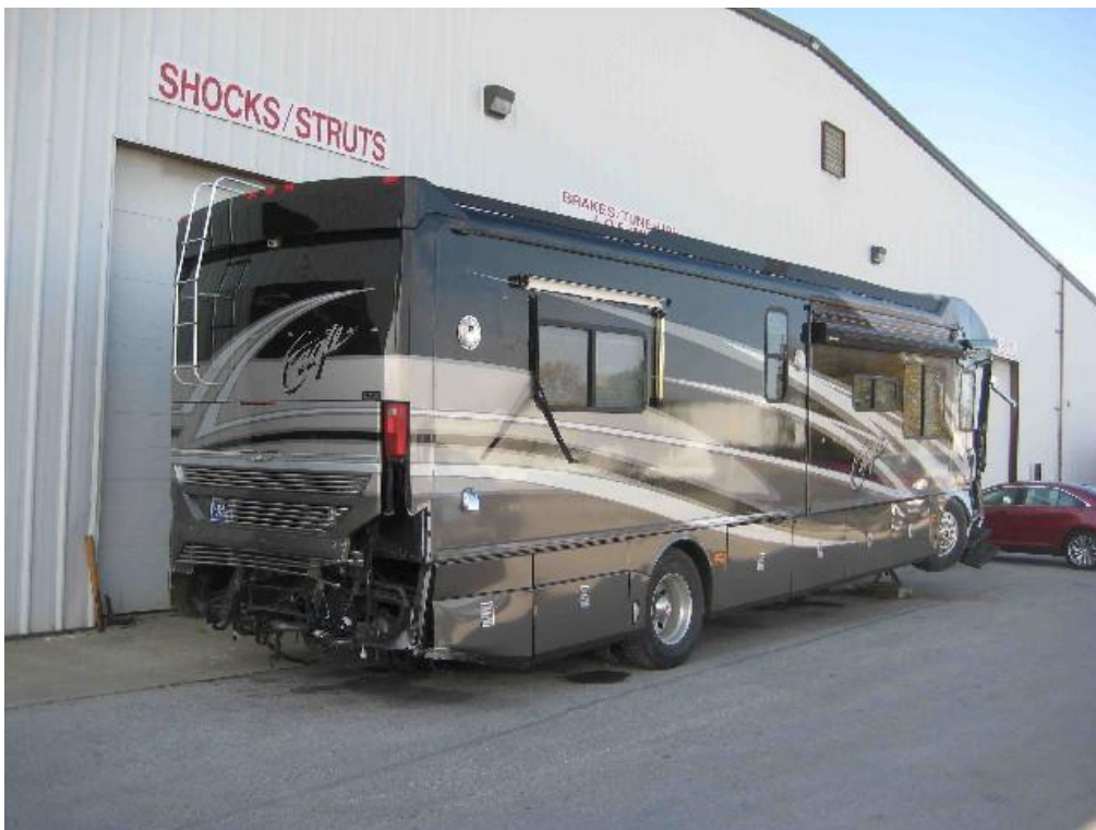
Figure 5: Rear overhang damage due to discontinuity between slope and basin bottom
