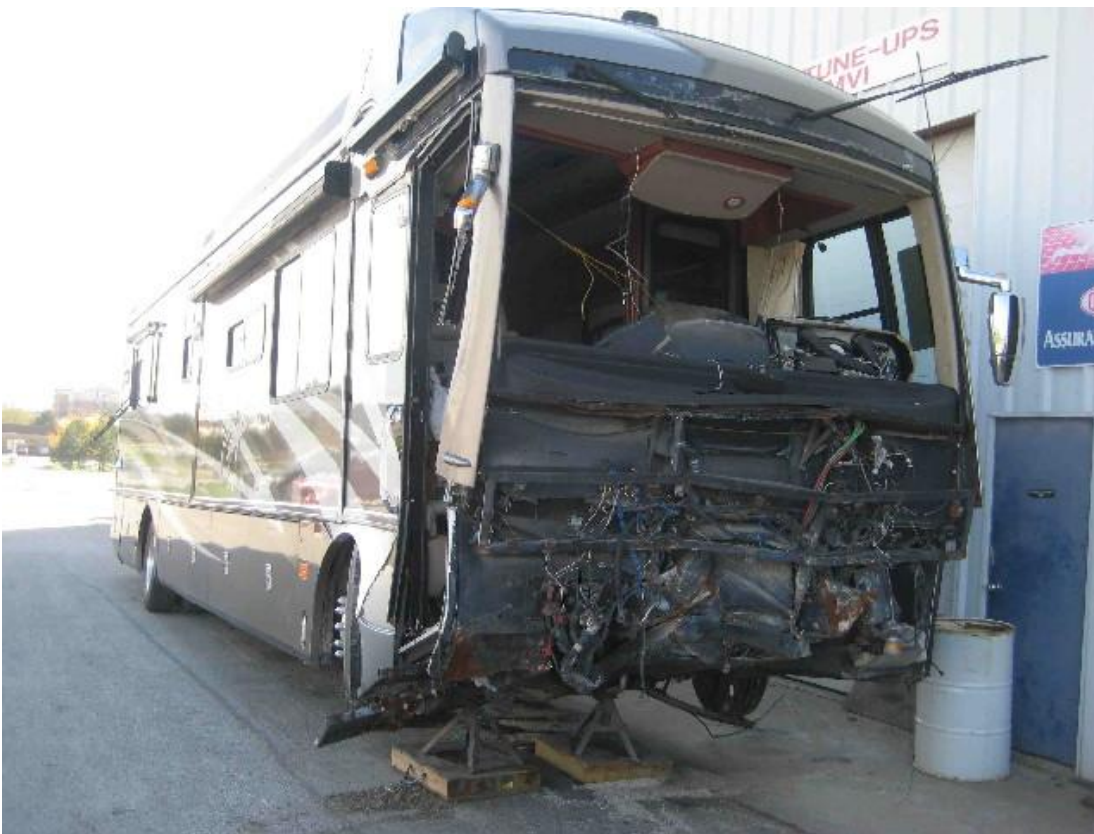
Figure 4: Front damage on motorhome due to impact with cliff face
