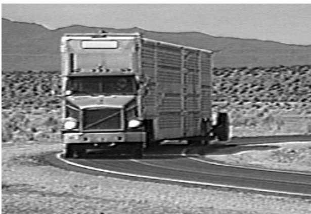
Figure 7. Screen capture from NATC videotapes showing the constant radius “constant velocity” maneuver
