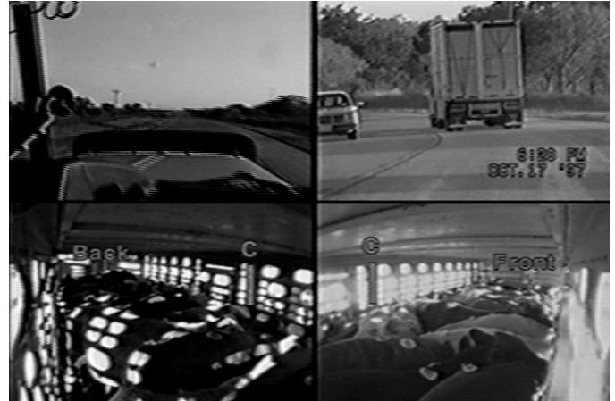
Figure 12. Screen capture from highway testing showing views of the cattle coordinated with a cab view and an external view
