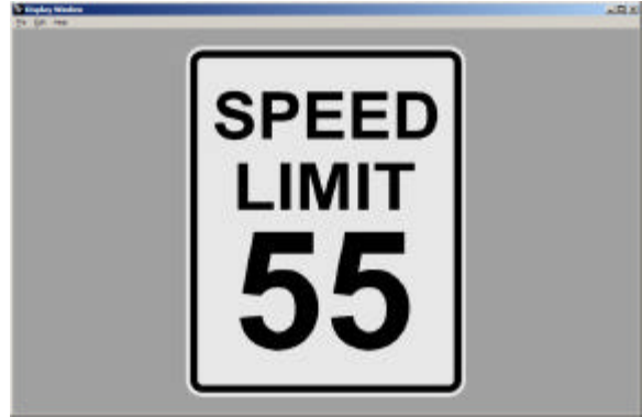
Figure 12. The text on this speed limit sign are surfaces created with the TextObject command. They are based on the Arial Bold font.
