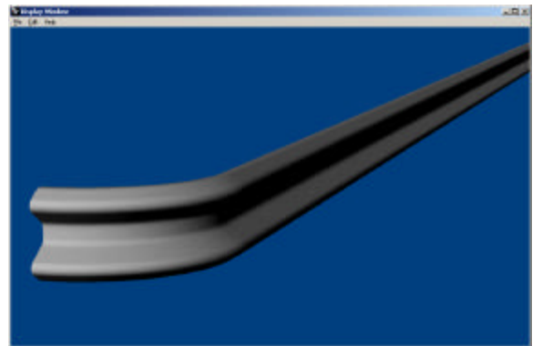
Figure 10. The guardrail was constructed with the Sweep1 command. A rail curve establishes the curved path of the guardrail.
