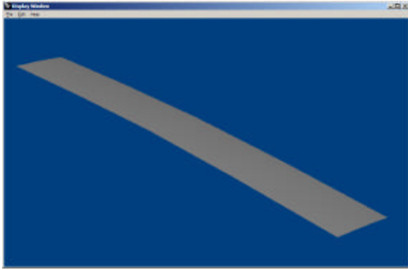
Figure 2. A surface created with the NetworkSrf command is smooth in both directions.
