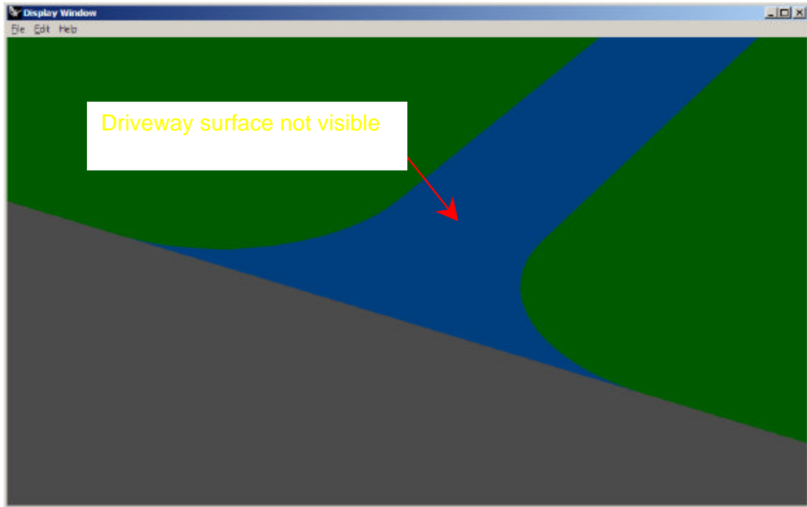
Figure 18. The surface normals of the driveway are reversed. With render backfaces disabled, the drive is not visible when rendered. The render background color shows through the surface.
