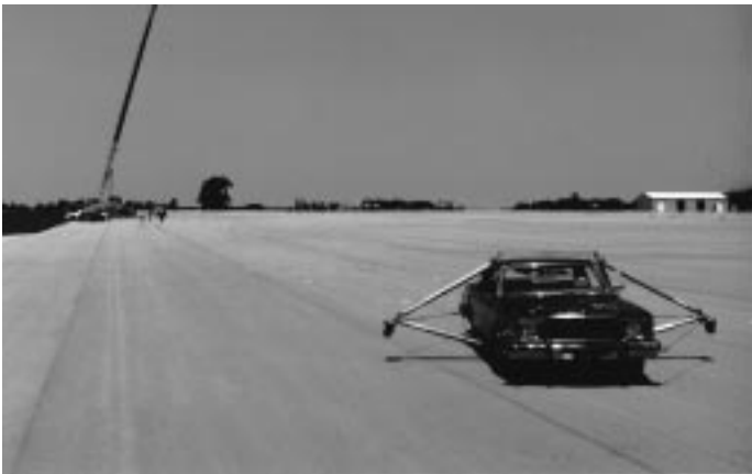
Figure 2 - Test vehicle, a 1976 Ford Granada 2-Dr Sedan, fitted with outriggers.
